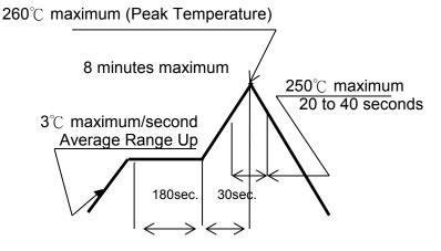
(Preheat Temperature预热温度: 150~200℃ Maximum.) Temperature Condition Graph.温度状态图 (Temperature on Board Pattern Side )
