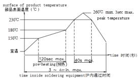
9 Automatic Flow Soldering (自动焊接)
